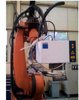
The laser welding systems: (a) 2kW fiber laser (left): 2.5-axis gantry machine with IPG YLS-2000 (2.0mm*mrad beam quality), (b) 6.6kW disk laser welding system (right): 5-axis KUKA robot with TRUMPF TruDisk6602 (8.0mm*mrad beam quality)
