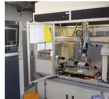
The laser welding systems: (a) 2kW fiber laser (left): 2.5-axis gantry machine with IPG YLS-2000 (2.0mm*mrad beam quality), (b) 6.6kW disk laser welding system (right): 5-axis KUKA robot with TRUMPF TruDisk6602 (8.0mm*mrad beam quality)
